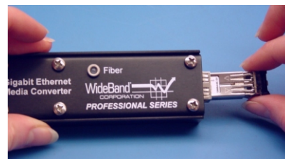
Loading a Mini-GBIC into the Media Converter
